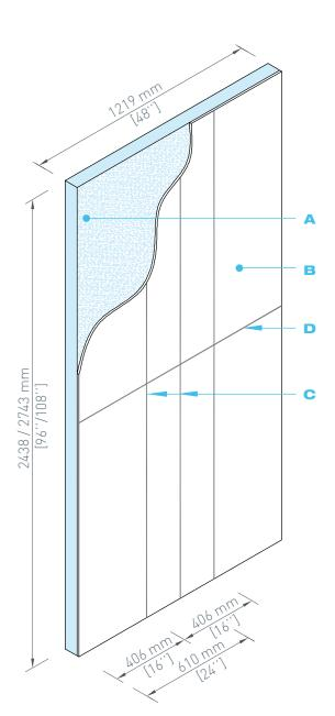
The **OSB.Comfort**™ boards manufactured by Styro Rail™ are composed of type 2 expanded polystyrene [EPS] rigid insulation laminated to an oriented structural board [OSB]. They comprise of perforations for complying with permeability requirements.
