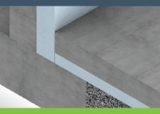
100% continuous insulation between the foundation wall and the slab. No thermal break.
