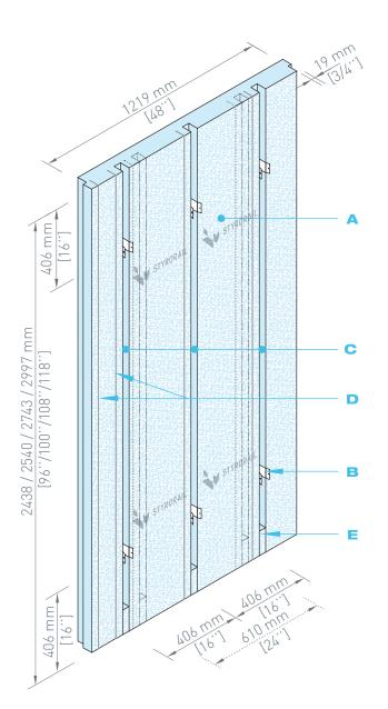
The **SR.2X4**<sup>™</sup> panels manufactured by Styro Rail<sup>™</sup> offer an alternative to traditional insulation of basements walls. They are produced in type 1 expanded polystyrene [EPS] rigid insulation. Each panel is comprised with grooves at every 406 mm [16"] o.c. or 610 mm [24"] o.c. in order to facilitate the insertion of wood stud framing. Metal brackets are provided to firmly secure the wood stud framing to the concrete wall.
