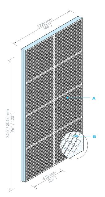
The **SR.Drain**<sup>™</sup> panels manufactured by Styro Rail<sup>™</sup> are composed of type 2 [200 series] or type 3 [300 to 600 series] expanded polystyrene [EPS] rigid insulation. They comprise of a smooth surface and a surface with diamond a shaped pattern allowing water to drain downwards.
