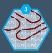
Spacing at 3", 6", 9", and 12", without the use of wire mesh to hold the pipes in place.
