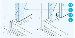
Vapor barrier underneath the furring strips
