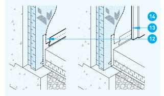
Vapor barrier underneath the furring strips
