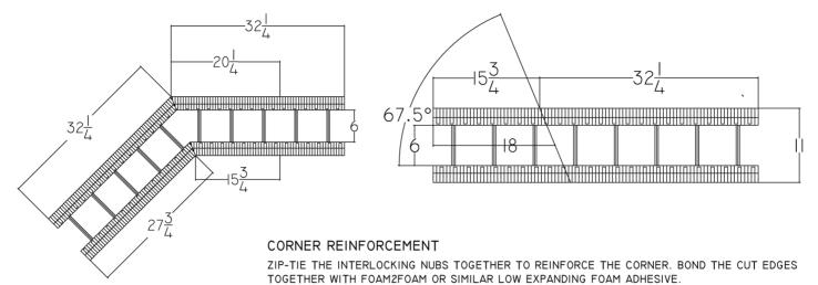
ADEQUATE BRACING AND STRAPPING IS REQUIRED FOR ALL FIELD FABRICATED CORNERS. LARGER BLOCK CORES REQUIRE ADDITIONAL BRACING AND STRAPPING ON OUTSIDE CORNER CUTS. CONTACT BUILDBLOCK TECHNICAL SUPPORT FOR MORE INFORMATION.
