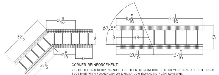
ADEQUATE BRACING AND STRAPPING IS REQUIRED FOR ALL FIELD FABRICATED CORNERS. LARGER BLOCK CORES REQUIRE ADDITIONAL BRACING AND STRAPPING ON OUTSIDE CORNER CUTS.
