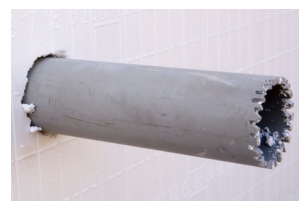
Figure 7.1.3 Cut small teeth on one end of the pipe sleeve and use to saw through the other side of the block to create a smooth opening.
